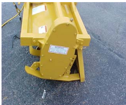
Side Gear Drive with Heavy Duty Casting Cover Heavy Duty Casting Cover Side Gear Drive
